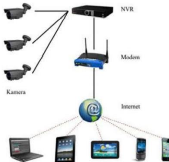
Figure 4. IP Camera CCTV system
